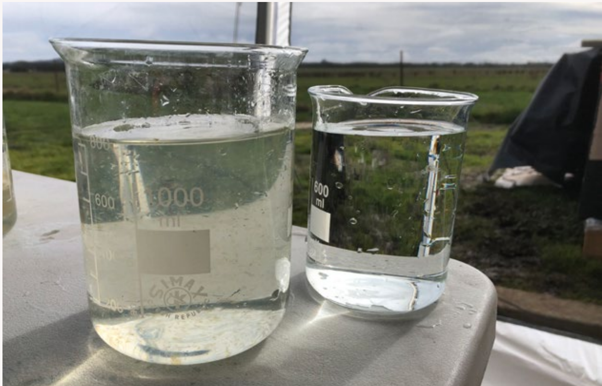
Figure 7. Recycled water before and after passing through the ceramic ultrafiltration membranes
